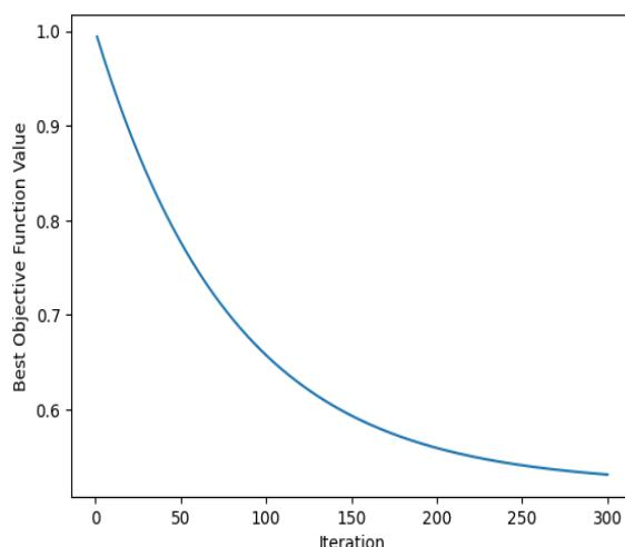
Figure 8 shows the stable convergence of the AMDE-PSO hybrid algorithm, with a steep initial decline in the objective function (broad exploration) followed by a gradual flattening in later stages (local exploitation). The smooth trajectory without severe oscillations and the final stabilization of the objective value confirm an effective exploration-exploitation balance and a reduced likelihood of entrapment in local optima.
