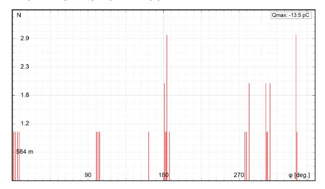
Quantitative evaluation of the key PD indices reinforced the visual PRPD analysis. As the artificial contamination on the surface increased, the apparent charge (Q) of discharges in ceramic insulators rose sharply, showing a step-like escalation once the pollution layer became conductive enough to support stronger surface breakdown. The repetition rate (n) also increased but tended to plateau as severe contamination promoted fewer but larger energy
